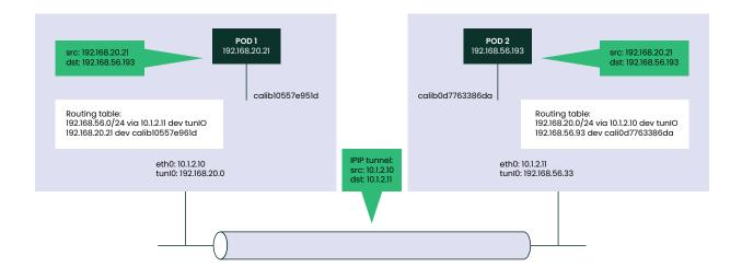
The above diagram shows how a packet traverses between pods on different nodes. In this example, the Calico CNI network plug-in is used. Every network plug-in has a different approach for how a pod IP address is assigned (IPAM), how iptables rules and cross-node networking are configured, and how routing information is exchanged between the nodes.
